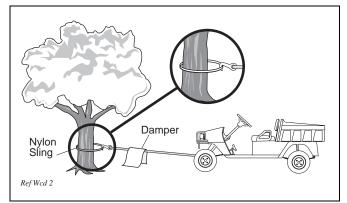
Fig. 7 Use a Nylon Sling and Install a Damper when Winching
